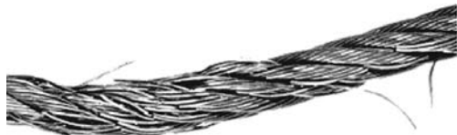
Fatigue (Undersized Sheave)
