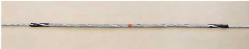
Reeving Splice Specifications
