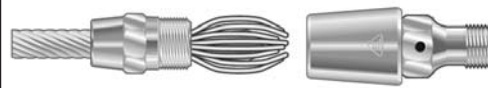
SLEEVE, PLUG & SOCKET: Plug driven in and strands closed to apply socket.
