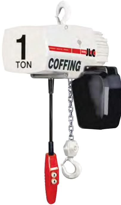
**COFFING JLC Models** - Designed for industrial duty performance. Compact in size, the JLC features a multiple disc motor brake, overload clutch and chain end stop for safety.
